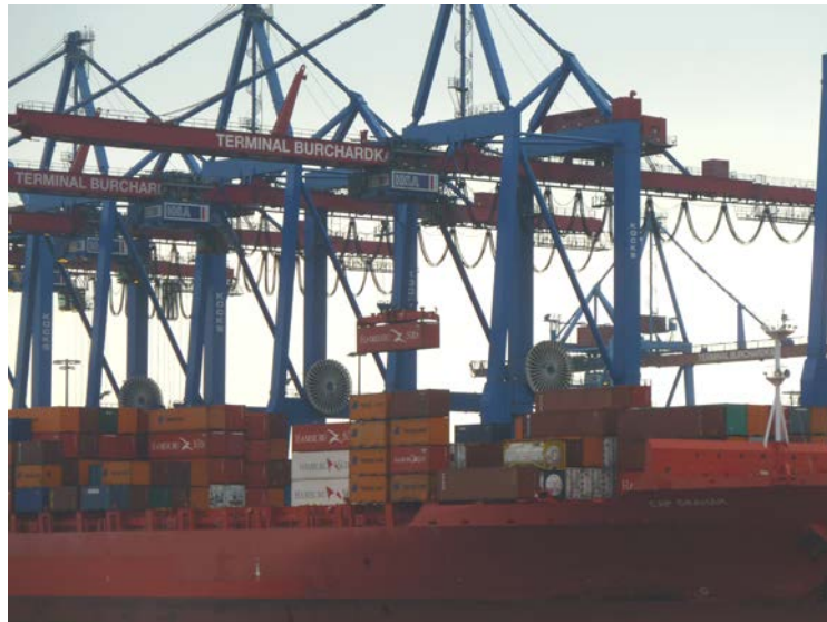
Picture 1: Ship-to-shore cranes
