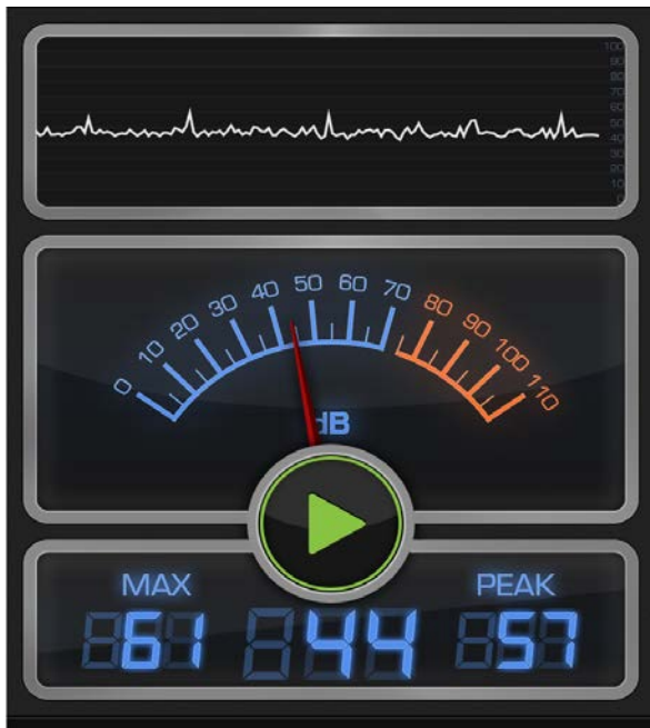
Figure 7 - Background noise recorded before starting the bandconveyor
