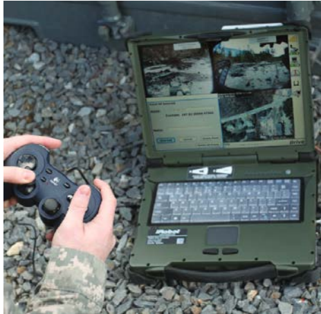
Fig.12 PackBot® 510 control system
