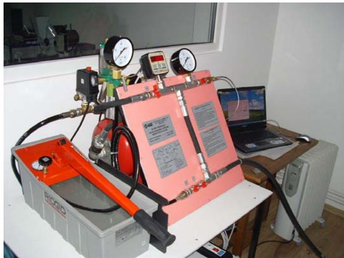
**Fig. 2.** Test stand for hydrostatic and cyclic pressure:
