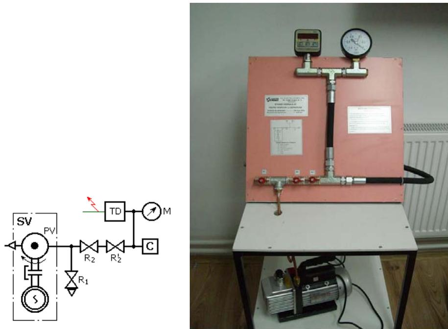
**Fig. 3.** Test stand for negative pressure: hydraulic diagram and view
