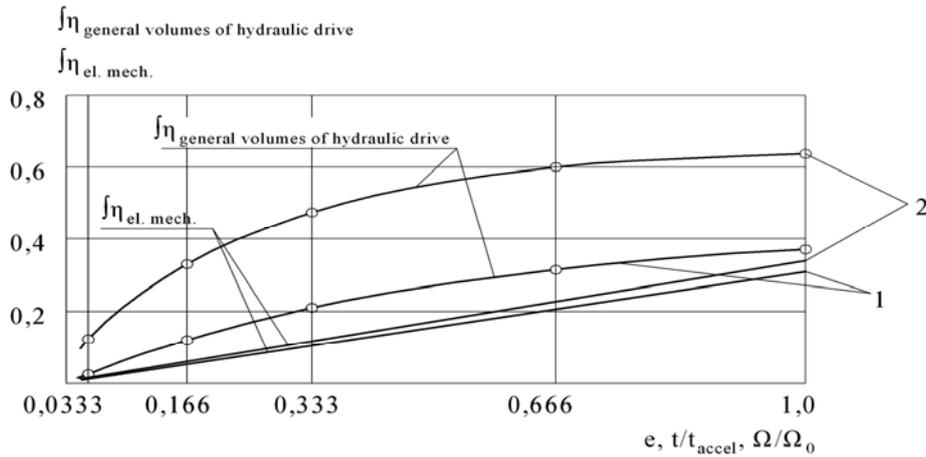
**Fig. 3.** Diagrams of dependency of the integrated coefficient of efficiency in the three-dimensional hydraulic drive and in the electromechanical drive with phase-wound rotor on  $e$  which is the regulation parameter (current productivity to nominal productivity ratio),  $t/t_{accel}$  which is relative time,  $\Omega/\Omega_0$  - relative velocity under different loadings 1, 2 ( $M_2 > M_1$ )
