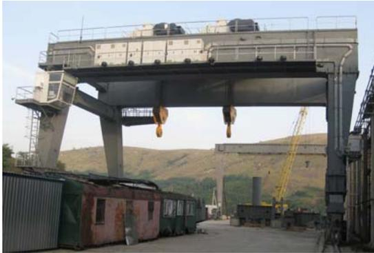
**Fig 5.** Portal bridge special-purpose crane with the load-carrying capacity of 420/420/16 t
