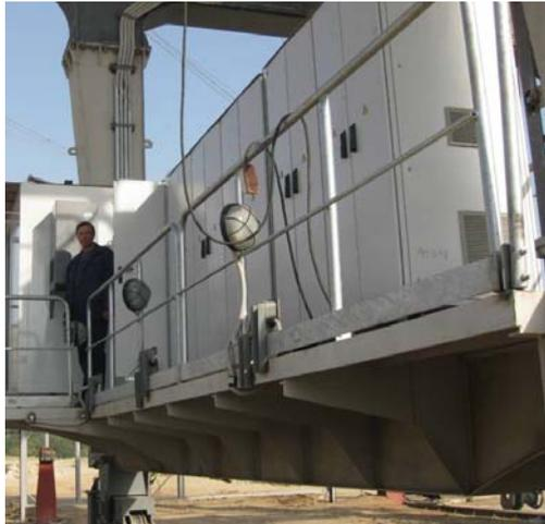
**Fig. 9.** Crane control device placement
