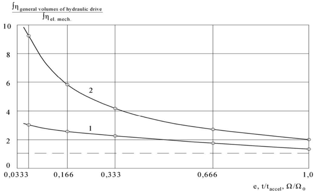
**Fig. 4.** Diagrams of dependency of  $\int \eta_{e2} / \int \eta_{eM}$  on  $e, t/t_{po32}, \Omega/\Omega_0$  with different loadings 1, 2 (the dashed line corresponds to  $\int \eta_{e2} / \int \eta_{eM} = 1, M_2 > M_1$ )
