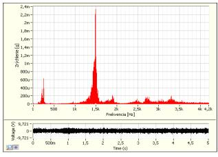
**Fig. 2.** Dependence of vibrations acceleration amplitude course at corresponding frequency on the lineness of abrasive mesh 50 at speed of technological head feed 50 mm min<sup>-1</sup> for the steel S335 JR (11 523)
