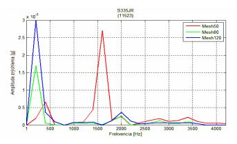
**Fig. 3** Comparing graph of vibrations acceleration amplitude courses at corresponding frequency for three researched dependences of abrasive at speed of technological head feed 50 mm.min<sup>-1</sup> for the steel S335JR (11 523)
