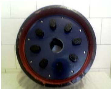
Fig. 8. Semicoupling 2 with brake sheave 7 (view on the left, right)
