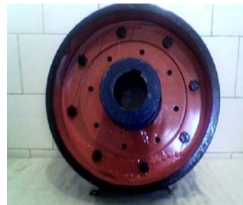
Fig. 8. Semicoupling 2 with brake sheave 7 (view on the left, right)
