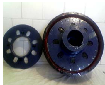
Fig. 5. Assembly coupling and retaining disc 5
