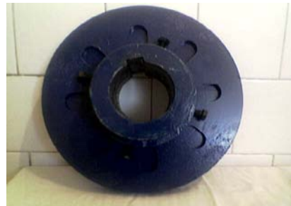
Fig. 7. Semicoupling 1 with restraining disc 5 mounted
